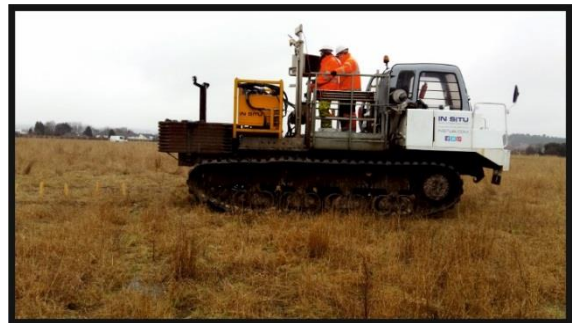
Figure 4. Photograph of the 15 tonne Morooka based tracked CPT rig undertaking the probehole fissure investigation
